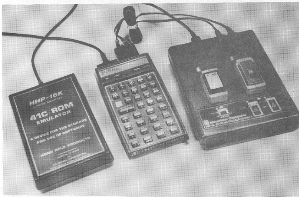
Figure 12 — EPROM burner, right from Mountain Computer. MCODE in the EPROM box burns EPROMs in a few minutes.
