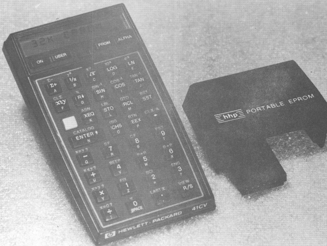
Figure 14 — State-of-the-art in small size large capacity EPROM memory. The Portable EPROM from Hand Held Products was announced August 15, 1983.
