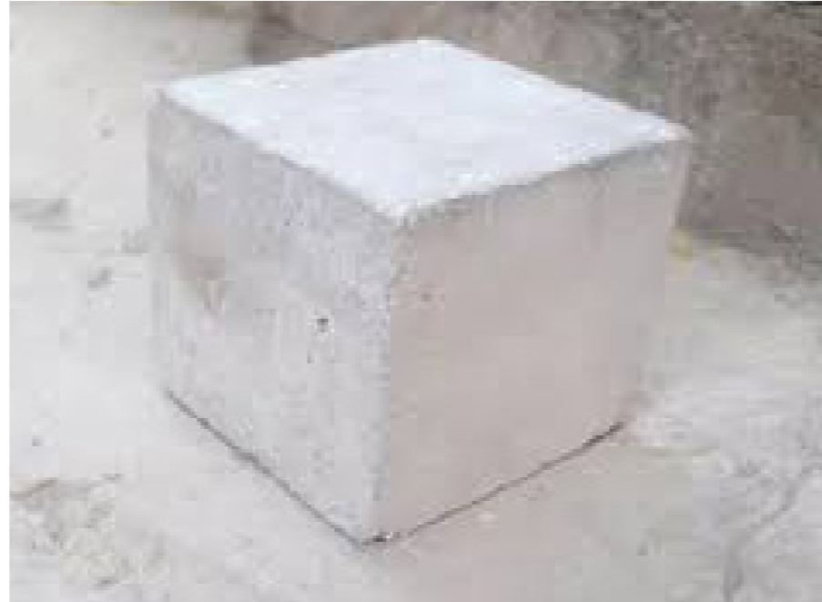
REDUCED CARBON CONCRETE SPECIFICATION By using GGBS addition to the concrete mix
