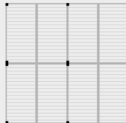
Duplex pergolas sharing columns
