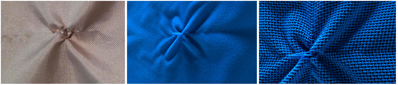
Figure 9: Middle: Snag formed by pulling two yarns while blocking the outward motion of the cloth. Left: Real snagging under similar conditions. Right: Close-up of the snag. We encourage the reader to zoom in to fully appreciate the details, such as rendered yarn torsion.
