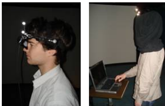
Fig. 1 The experimental apparatus. Left: the participant wearing the HMD and the tracking equipment. Right: the participant equipped and wearing the opaque fabric in front of the table with the laptop computer.
