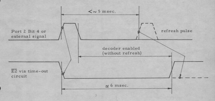
When Port 2 Bit 4 is configured in the input mode and the external column enable signal is selected, it is possible to use the latter signal as a data ready indicator by connecting jumpers 5-6-7, and software scanning Port 2 Bit 4.
