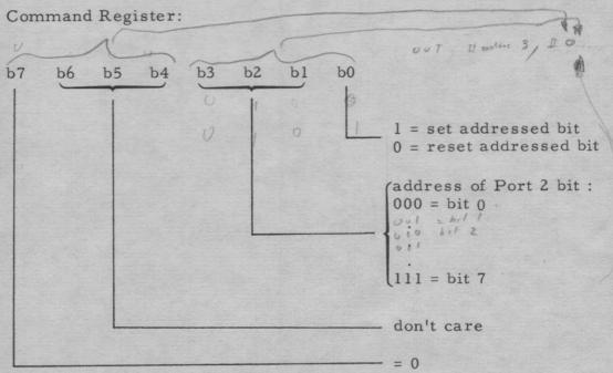
The following software example will set RIC Port 2 Bit 3 of a RWC module with address select switch set to 'E':
