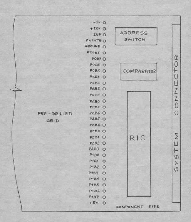
Figure 7.2.2 : Positioning of Available Signals on RWC-F
