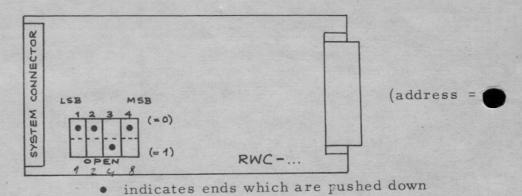
Note: In case the markings on the DIP switch are different from those mentioned above, the rockers must be set to the corresponding positions as indicated in the diagram above.
