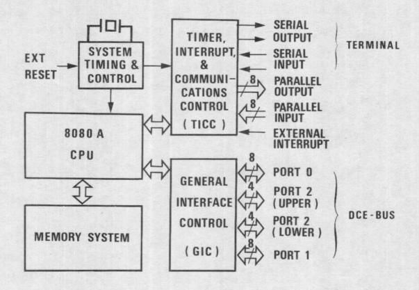
Figure 1-1. General DCE Processor Block Diagram for 8-bit Microcomputers
