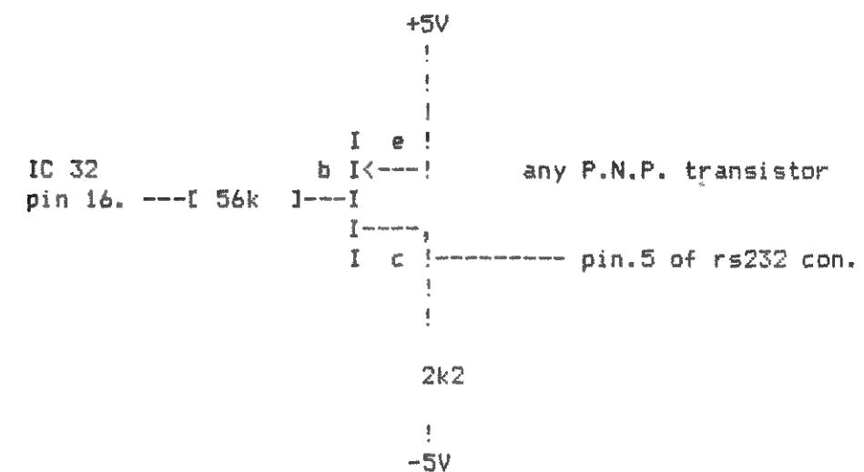
You could test the program by connecting 2 DAI pc with the rs232 connected:
